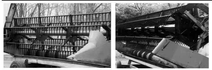
\*Strongest Reel Available \*Fingers use the patented "Gentle Finger" design. \*Fingers are guaranteed one year against breakage. \*Replaces Wood Bat Reels, Tear Drop Reels, and OEM Pipe Reels. \*Comes with all new bearings and hardware.
